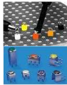
Test Points/ Terminals
